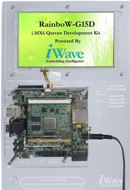
The Development Platform incorporates Qseven compatible i.MX6 SOM which is based on Freescale's i.MX6 Series multimedia focused processor and Generic Qseven compatible Development Board. This platform can be used for quick prototyping of any high end applications in verticals like Automotive, Industrial & Medical. Being a nano ITX form factor with 120mmx120mm size, the board is highly packed with all necessary onboard connectors to validate complete i.MX6 CPU features.
